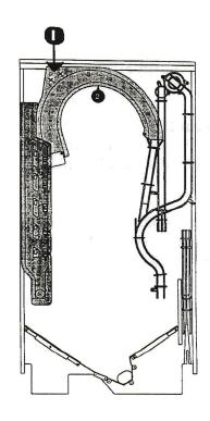
WE'VE DISCOVERED A POTENTIAL BALL HANG-UP AREA ON "POPEYE". PLEASE REFER TO THE PLAYFIELD DRAWING ON THE LEFT. TO CORRECT THE HANG-UP ADD 2 POSTS (PART # 03-8319-10) AND SCREWS\* (PART # 4108-01001-26) WHERE THE 2 X'S ARE IN ITEM 1. ITEM 1 IS ON THE REAR OF THE RAMP ASSEMBLY (ITEM 2) WHICH IS UNDER THE MINI-PLAYFIELD. LIFTING OF THE MINI-PLAYFIELD IS NECESSARY TO BE ABLE TO INSTALL THE NEW POSTS. ATTACHED TO THIS BULLETIN IS THE PROCEDURE FOR LIFTING THE MINI-PLAYFIELD. IT IS A
